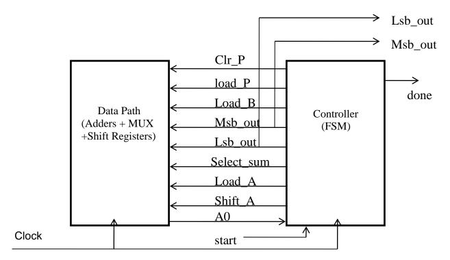
Figure 3. Data and control parts of the proposed architecture
