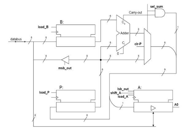
Figure 4. Proposed architecture of sequential multiplier
