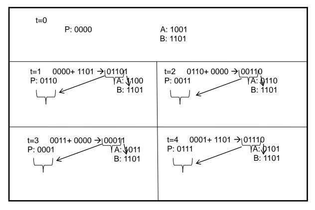
Figure 1. Hardware oriented multiplication process
