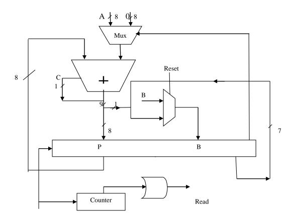
Figure 2. Conventional sequential multiplier
