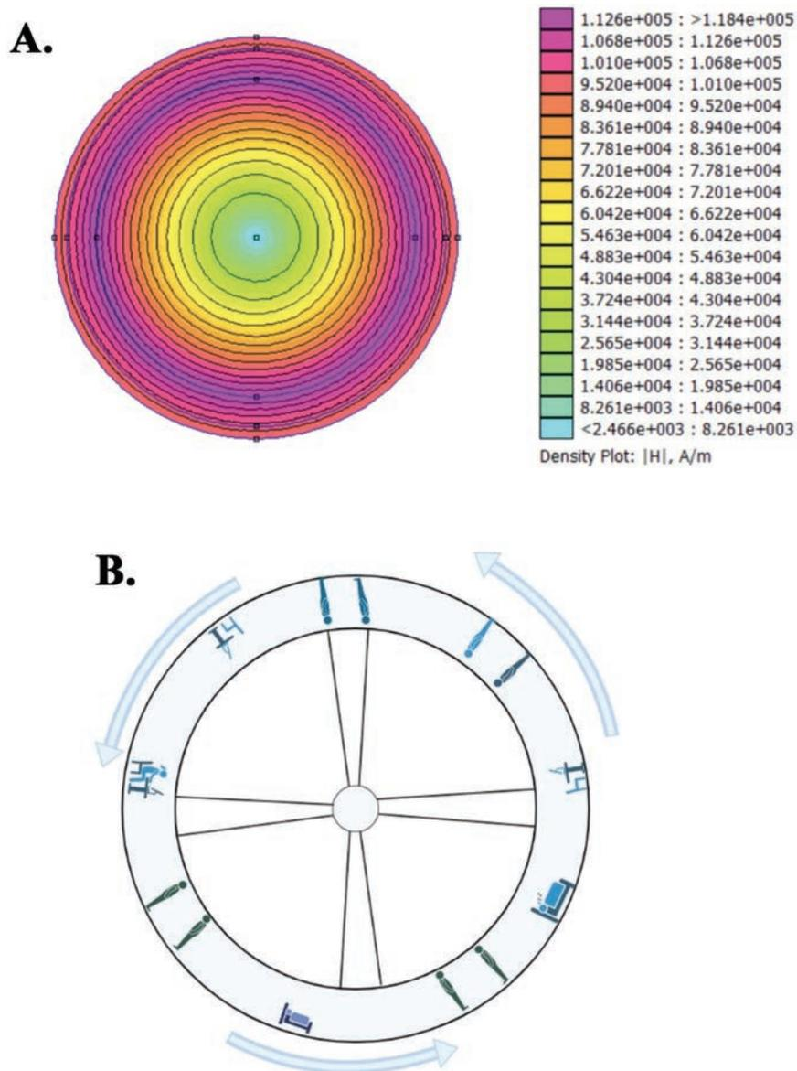
**Figure 3** One Coil Field Intensity and centrifugal force. **(A)** This image shows the intensity of the magnetic field in Amperage per meter. The actual coil's radius is the 2nd prominent dot from the middle to the outer dot. This was simulated through the FEMM simulation software. **(B)** Centrifugal force can create artificial gravity by rotating the outer part of a spaceship around an axis.
