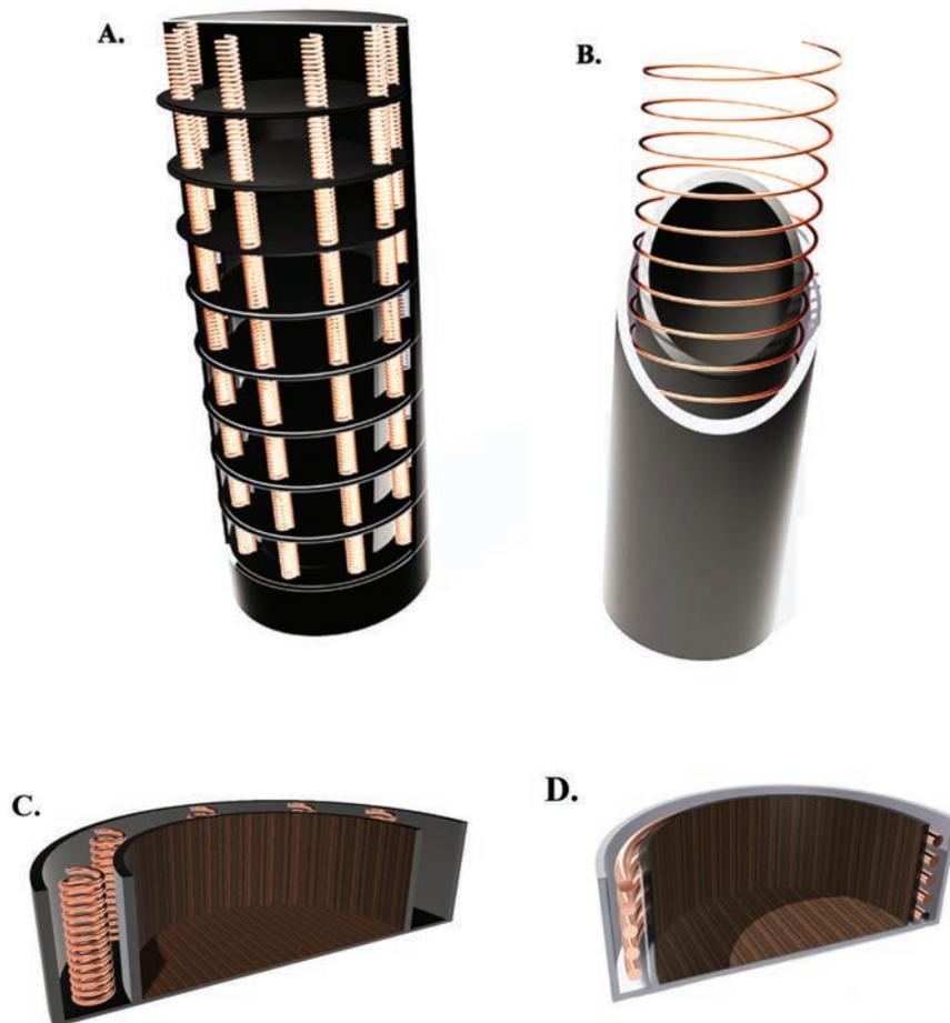
**Figure 1** 3D Model of 1- and 10-coil generator. (A) Shows how the coil's arrangement would be placed in a 10-coil system. (B) Image depicts 1-coil arrangement. This model favors height over length/width for a spacecraft/module. (C) Image depicts a smaller version of the 10-coil arrangement made for 1 floor. (D) The image shows the coil's arrangement in a one coil system. This model is most useful in more mainstream spaceships.
